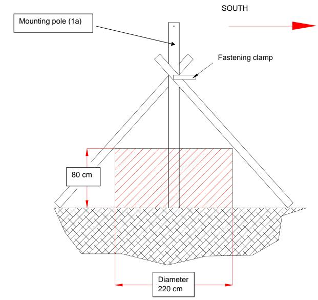
fig. 4.1 Dimensions of surface foundation
