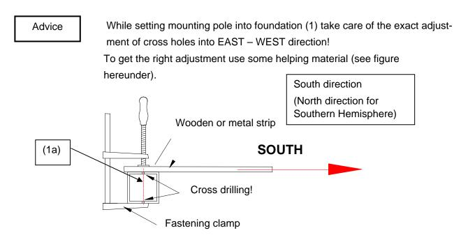
During drying-procedure of foundation please use wooden boards to support mounting pole. In case of installation on flat roofs, stability can be effected with clamping belts.
