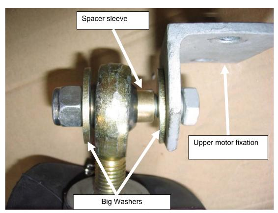
Assembly of the upper motor fixation for actuators with spacer sleeve.
